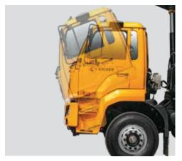
Fully suspended cabin with hydraulic tilt mechanism
